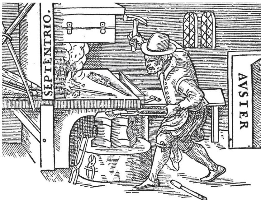
Figure 1. Making magnets by hammering hot iron in the meridian.<sup>1</sup> ‘Auster’ and ‘Septentrio’ come from an early scheme of naming cardinal points from the winds: they correspond to north and south, respectively.
