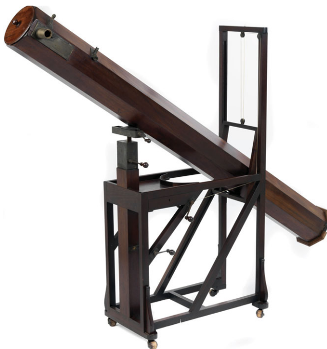
Figure 3. A Herschel 7-foot reflector. (Object number AST0960, image ID F5601-001; copyright © The National Maritime Museum, London.) (Online version in colour.)
